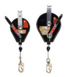
Self-retractable arrester with built in two-way rescue/ recovery mechanism. Fall arrest device with rescue lifting and lowering facility, equipped with a recovery mechanism operated by a device mounted handle. After an arrested fall, or if the user becomes incapacitated at the bottom of a shaft, the recovery mechanism can easily be engaged by a second person to raise or lower the person to a place of safety.
