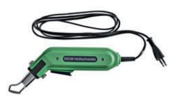
Ideal machine for cutting the ropes and accessory cords. Compact hand-held. The blade heats quickly. For save and fast cutting the ropes.
